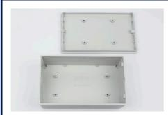
The PCB is supported around the perimeter of the base by card edge supports. Size 3 & 4 also have four half board central supports (which can be removed to make way for solder points on the bottom of your PCB).
